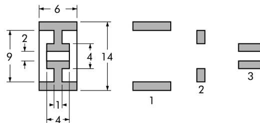
A steel flywheel is sectioned into three different hollow cylinders; the rim, webbing and hub. Calculate the WK<sup>2</sup> of parts 1, 2, and 3; then add for the total WK<sup>2</sup> as shown.
